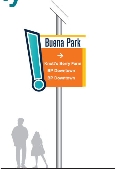
(S3) Vehicular Directional Sign (mounted to existing pole)
