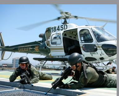
Position System (GPS), a Public Safety Radio System for communications with all regional police and fire agencies and a complete public address/siren system. Aircraft have a maximum speed of 155 knots, a maximum range of 350 miles, can stay in the air for 3.5 hours, have a takeoff weight capacity of 4961 pounds, and can hold six personnel.
